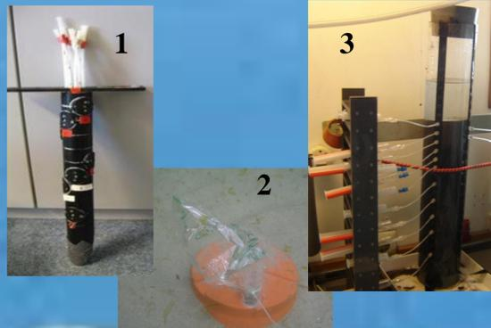
Fig. 3 Groundwater sampling via 1) piezometers, 2) seepage meter, 3) rhizons.
